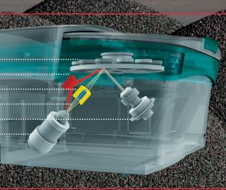
Unique binary-alloy anode emits palladium excitation radiation that gives best results for sodium to chlorine, iron to molybdenum, and hafnium to uranium, while emitting cobalt excitation radiation for potassium to manganese. It's like having two tubes in one instrument!
