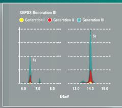
Three generations of SPECTRO XEPOS: sensitivity trending ever upward
